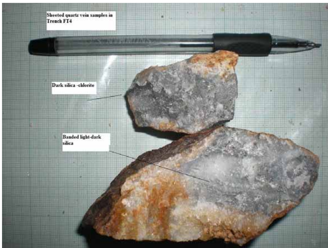
Figure 5. Banded dark silica-chlorite and possible ginguro ore textures, assayed 59g/t Au, 154g/t Ag in character-sampling of sheeted veinsets in FT4 (a zone of 4m at 10.04g/t Au)
