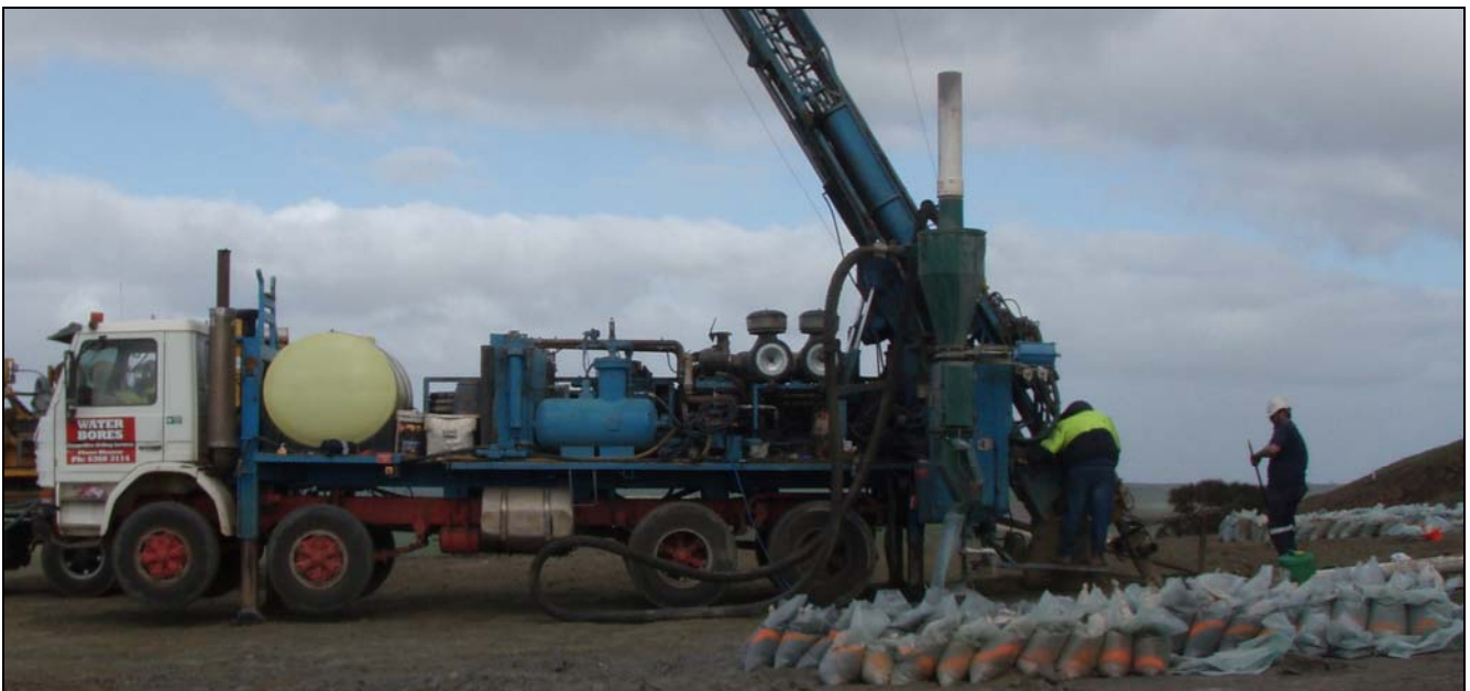
RC Drill rig operating at the O'Neil Zone
