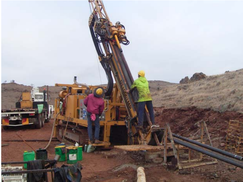
Track Mounted Diamond Rig Working 10km to the west of Cambrai
